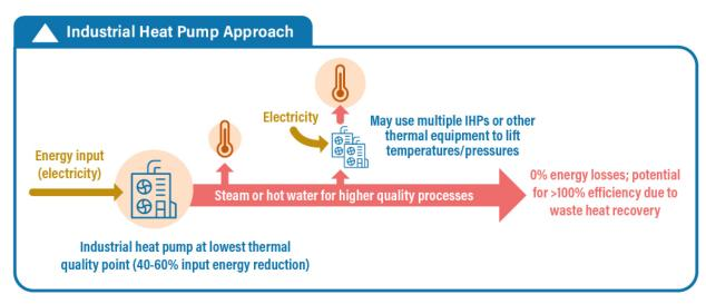
Orange circles show "size" or level of thermal quality of thermal load (large = high thermal quality load, small = low thermal quality load)
