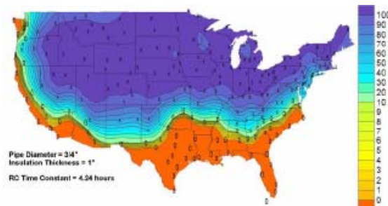
Figure 1. Probability of at Least One Pipe Freeze in 20 Years (assuming house is always occupied) Source: DOE 2005
