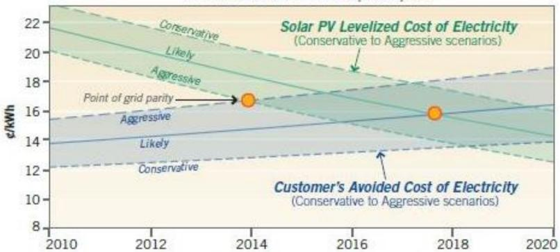
PV cost/performance typical for the Northeast US; Debt 8% equity 10% (80:20), 10 yrs debt, 25 yr lifetime, 30% ITC (assumed beyond 2016); includes state incentives; 2010 electricity costs are typical for Northeast states with EIA electricity escalation rates.
