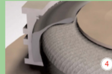
The mold is heated with steam in order to provide the heat necessary to cure the tire.
