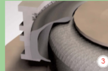
The tread pattern and lettering on the sidewall of the tire are created.
