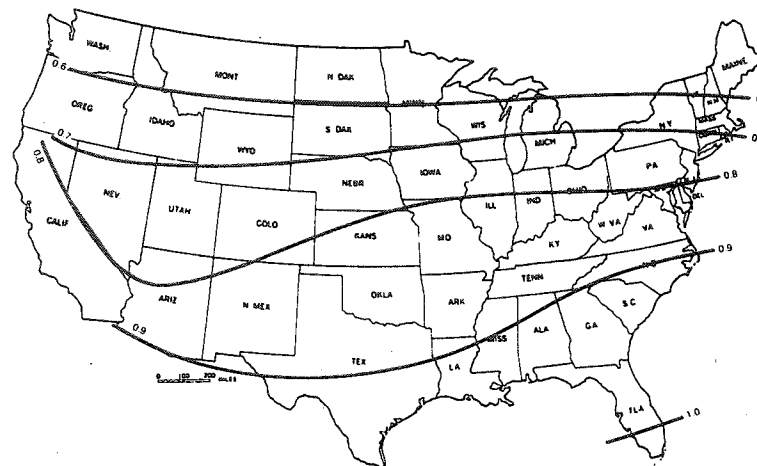
Fig. 6. Ratio of the SEER to the rated EER for properly sized air conditioning units.
