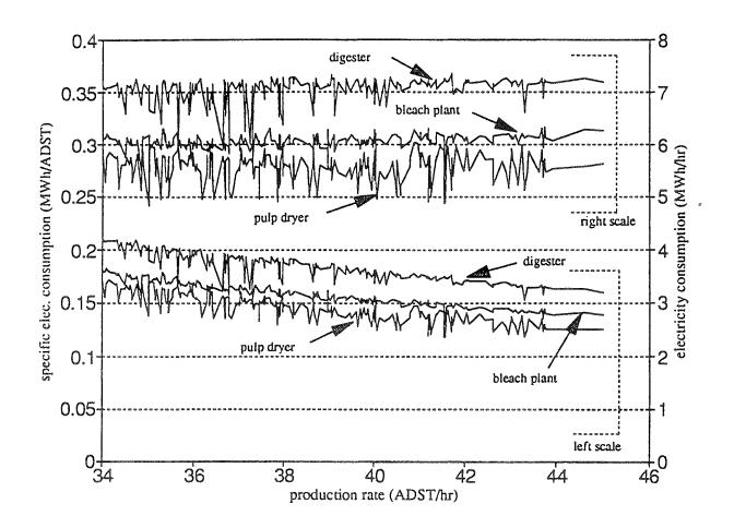
Fig. 3.6. Power demand in digesters, bleach plant, and pulp machine for a U.S. kraft pulp mill (Subbiah et al., 1995). Power demand in digesters is dominated by pumps, in the bleach plant by pumps and mixers, and in the pulp machine by fans and vacuum pumps.
