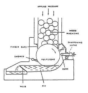
Fig. 2.6. Grinder for stone groundwoood (SGW) pulp production (Eliah and Lowitt, 1988). A recently sharpened pulpstone gives a coarser pulp, so a SGW pulp mill typically has many units from which the pulp is mixed to maintain uniform quality.
