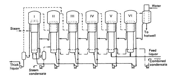
Fig. 3.2. Sample multiple effect evaporator sequence (Grace, 1989b).
