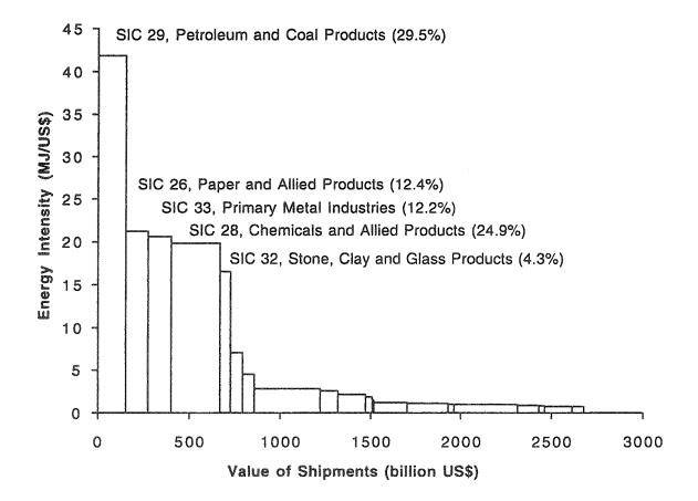
Fig. 1.1. Energy intensity for different industry groups at the 2-digit SIC level plotted against the value of shipments in 1991. Numbers in parentheses are percentages of total manufacturing energy consumption (MECS, 1994; ASM, 1992).
