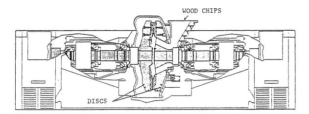
Fig. 2.7. Double disc refiner (Borg, 1989). The gap between the discs at the periphery is only about 0.1 mm. A refiner typically operates at 1500-1800 rpm.
