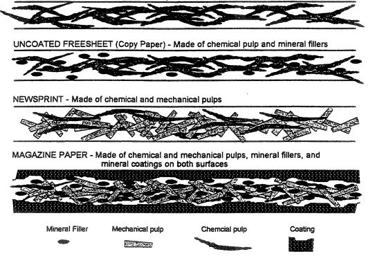
Fig. 2.2. Typical paper and paperboard compositions. Source: R.E. Buttner, H.A. Simons, Vancouver, BC, Canada.
