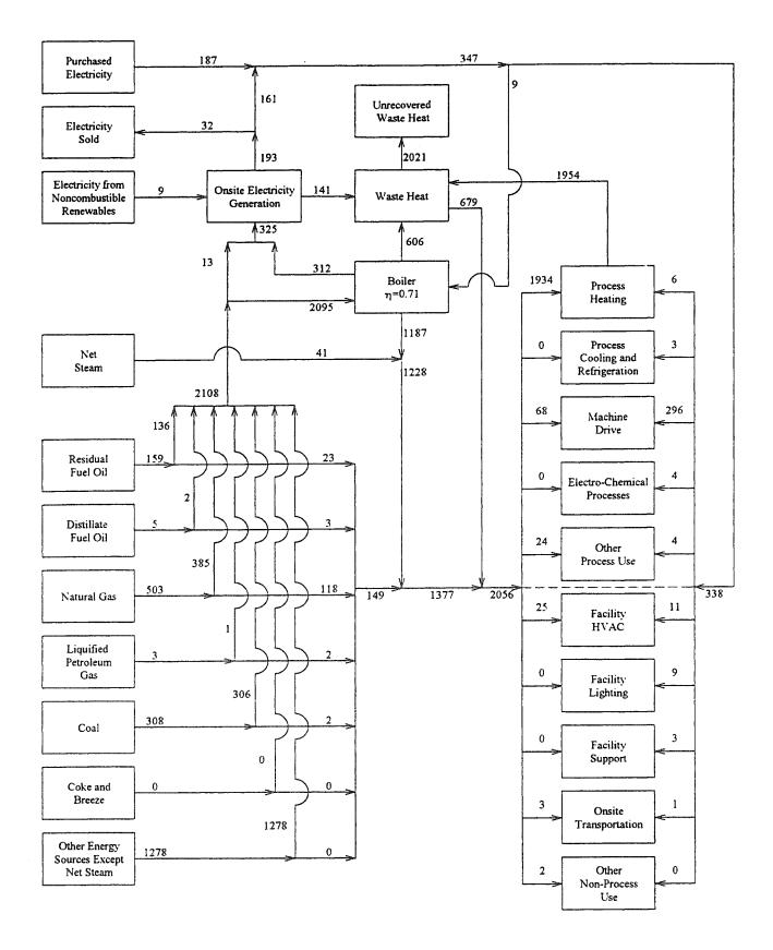
Fig. 1.4. Estimated energy flows (PJ per year) in the pulp, paper, and paperboard industry in 1991. Source: Barry Hyman, Dept. of Mechanical Engineering, University of Washington, personal communication, Seattle, WA, May 1995. See also Giraldo and Hyman (1994).
