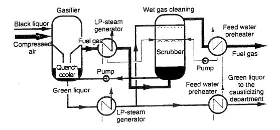
Fig. 4.3. High-temperature/smelt-phase, entrained-bed black liquor gasifier with quench (Kvaerner type) and wet gas clean up (Ihren, 1994). Pressurization of the gasifier facilitates recovery of heat at higher temperature and pressure.
