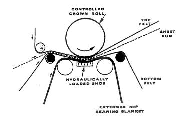
Fig. 3.4. Principle of the extended nip press (deBeer et al., 1993).
