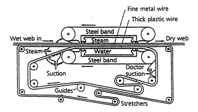
Fig. 3.5. Principle of the Condebelt drier (deBeer et al., 1993).
