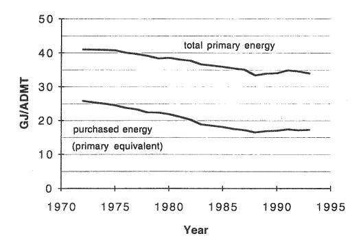
Fig. 1.3. Total primary energy and purchased energy use in the pulp, paper, and paperboard industry. Purchased electricity and steam have been converted to their primary energy equivalents using 10.8 MJ/kWh and an 85% boiler efficiency, respectively. Source: Lisa Wolfe, American Forestry and Paper Association, personal communication, Washington, DC, May 1995.
