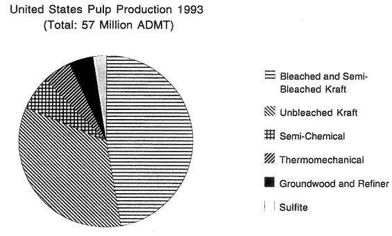
Fig. 2.1. U.S. pulp production by process in 1993 (AFPA, 1994a).
