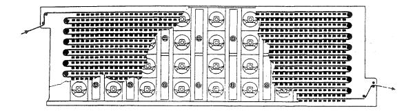
Fig. 3.1. An air float dryer (Perkins and Cowan, 1989). The pulp web moves over the dryer decks where hot air is blown to support the web and evaporate water. Turning rolls at the end sections move the web.
