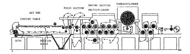
Fig. 2.8. Example of a papermachine with a single-wire wet end, and with both multicylinder and yankee cylinder drying (Borg, 1989).
