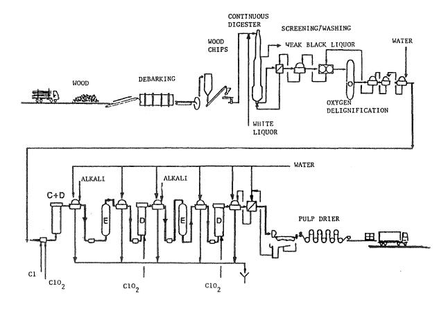
Fig. 2.4. Kraft pulping fiber line (Borg, 1989).
