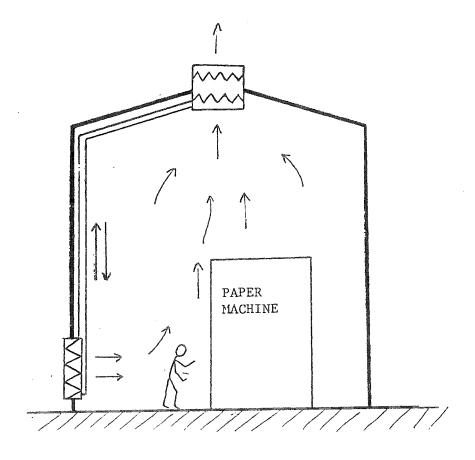
Fig. 3.7. Natural draft ventilation principle used in the paper machine area of a mill.
