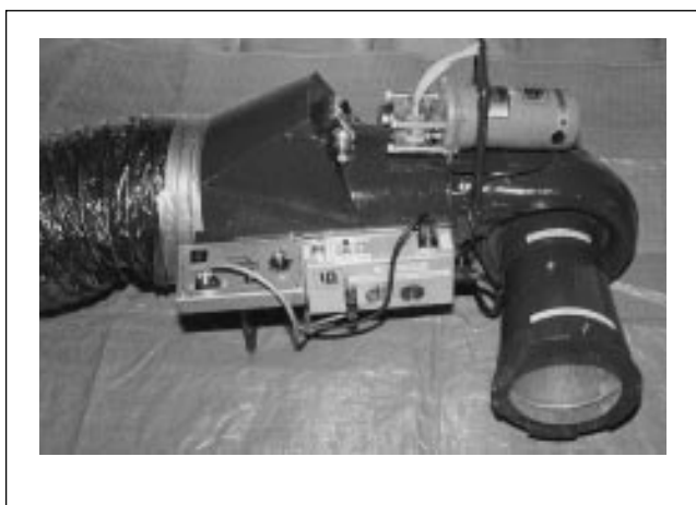
Figure 1. Aerosol injection apparatus used for the field study.
