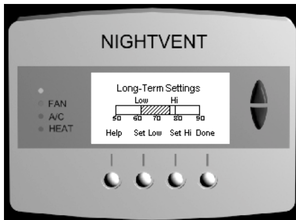
Figure 3. User Interface with “Long-Term” Cooling Settings Displayed
