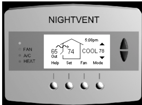
Figure 2. User Interface with Cooling Mode Screen Displayed
