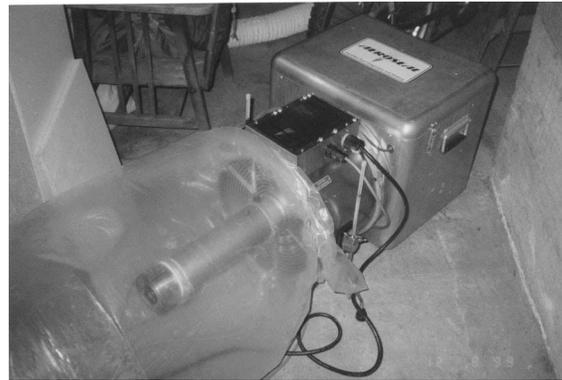
**Figure 2. The AeroSeal Tubing Connection**
