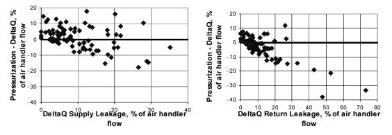
Figure 5. Change in Duct Leakage Flows Predicted by DeltaQ by Using Fitted Characteristic Pressures ( $l/s = cfm \times 0.47$ )
