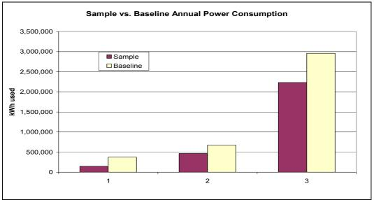
Note: 1 = Variable Primary Pumping, 2 = Free Cooling, 3 = High Efficiency VSD Chiller
