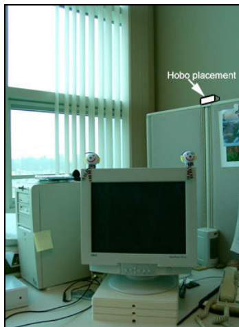
Figure 4. Hobo Placement on a Partition
