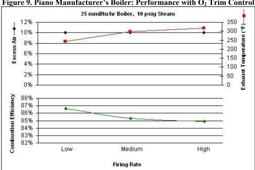
Figure 9. Piano Manufacturer's Boiler: Performance with O<sub>2</sub> Trim Control
