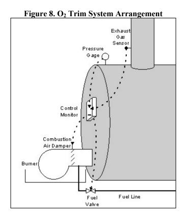
In addition to maintaining excess air at desired levels, O<sub>2</sub> trim eliminates the general safety protocol to calibrate excess air slightly higher than desired. For example, case 1 presented above showed low excess air at high fire, however excess air was still above the desired 10%. Excess air in the well-controlled case presented above, although low throughout the firing range, was also still above 10%. O<sub>2</sub> trim would allow for 10% excess air throughout the firing range.
