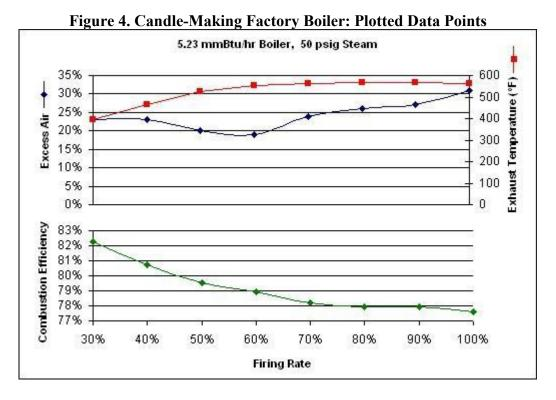
Note that exhaust temperature decreases at lower firing rates. This is due to combustion gasses moving more slowly through the boiler at lower firing rates, causing gas residence time within the boiler to increase. Increased residence time facilitates heat transfer, allowing each gas volume to exchange more heat and therefore exhaust at a lower temperature. In a well-controlled combustion air scenario, a boiler's combustion efficiency significantly rises at decreased firing rates.
