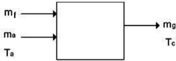
Figure 1. Mass Balance on Combustion Chamber
