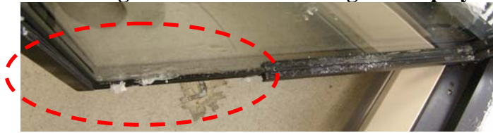
Figure 7. One Foot of Missing Gasket Used in Testing LT Display Case Leakage
