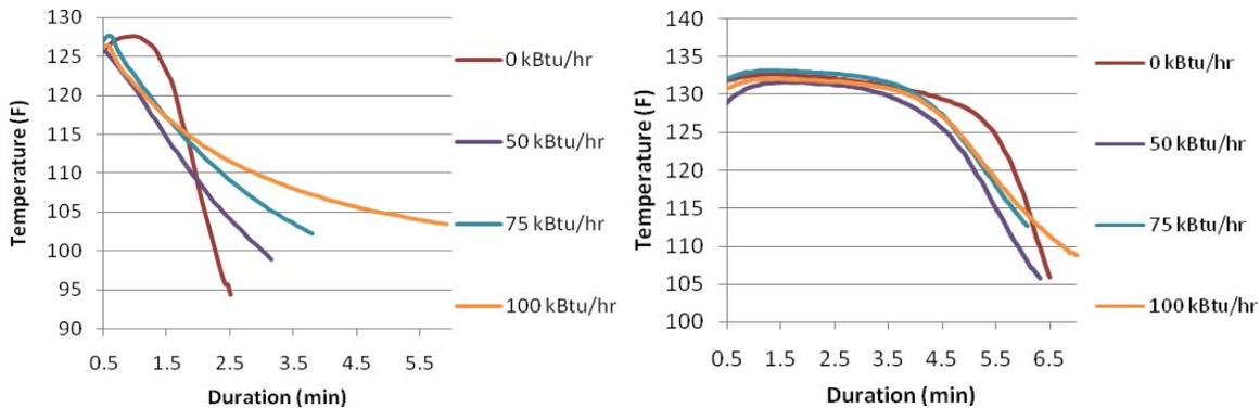
Note: 10 and 30 gallon HOT water heaters are left and right respectively. “0 kBTU/hr” refers to a no fire/pump draw.
