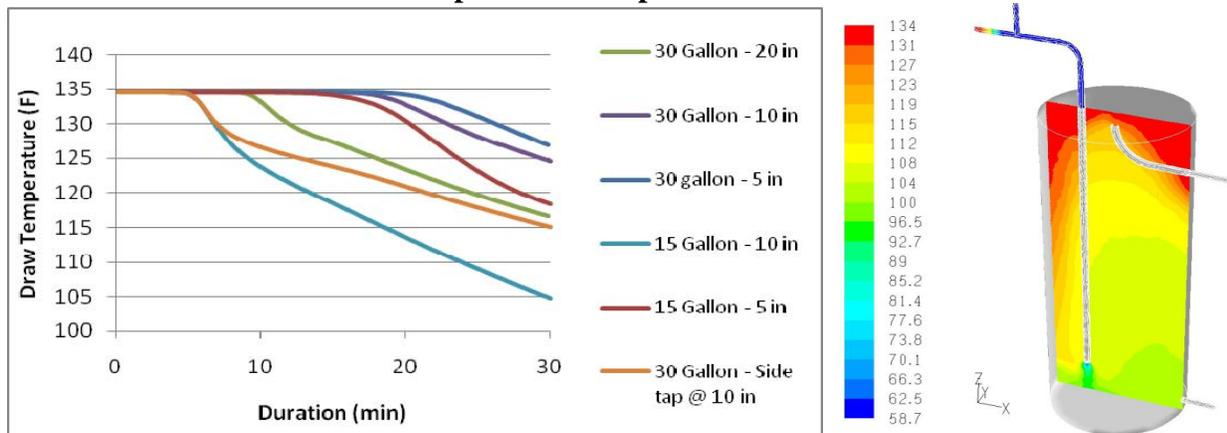
Notes: All temperature profiles are for diptubes terminating with various distances from the tank bottom unless otherwise indicated. CFD performed with FLUENT Version 6.3, example is 30 gallon tank with diptube 5" off tank bottom, after 15 minutes of the 0.5 gpm draw.
