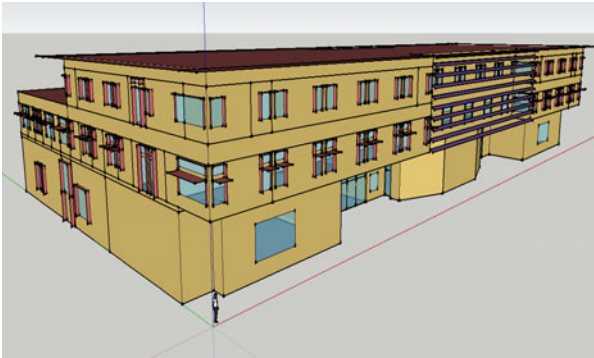
Figure 4: Model Representation of COB Showing Glazing and Overhangs.
