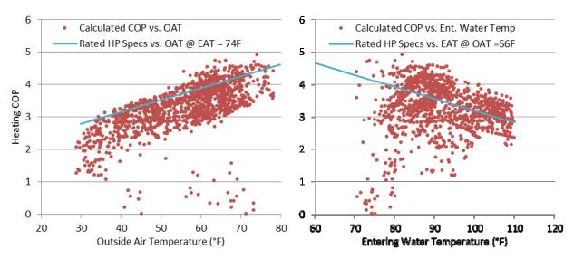
Figure 7. Measured COP for ASHP at Tucson house in space heating (a) versus outdoor air temperature (OAT) and (b) as a function of entering water temperature (EWT). Manufacturer-rated performance is also charted. (n=1,241 15-minute intervals).
