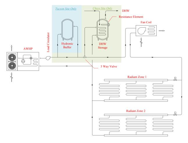
Figure 2b. Schematic of two alternate multi-function AWHP systems. Chico site includes DHW with electric resistance backup and three way valve to isolate hydronic load from DHW storage. Tucson site includes buffer tank in hydronic loop to decouple heat pump capacity from variable internal load.
