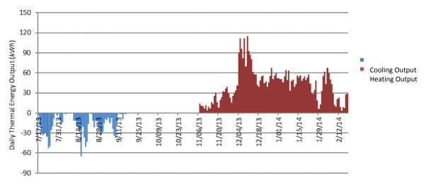
Figure 4. Daily thermal energy output (to the load circuit) for heat pump in heating and cooling.
