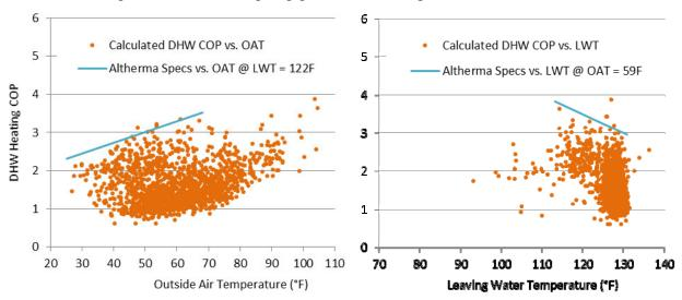
Figure 11. COP for the Chico AWHP in DHW mode as a function of (a) outside air temperature and (b) leaving water temperature. Manufacturer rated specifications are also plotted for each. (n = 1,607 15 minute intervals).
