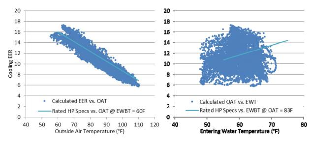
Figure 8. Measured cooling EER for ASHP at Tucson house as a function of (a) outside air temperature, and (b) entering water temperature. (n = 8,208 15-minute intervals) Manufacturer rated performance is also presented.
