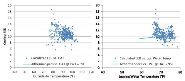
Figure 10. Cooling EER for the Chico house AWHP as a function of (a) outside air temperature, and (b) leaving water temperature. Manufacturer stated performance is also plotted. (n = 337 15-mminute intervals).
