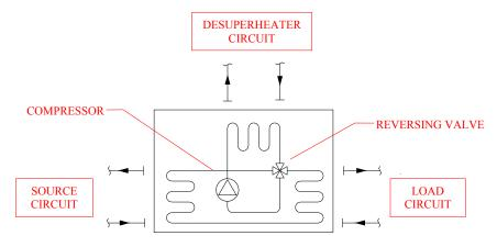
Figure 1. General schematic of a multi-function heat pump with desuperheater.
