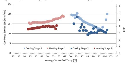
Figure 6. Average "Combined Service EER" for each mode of operation, as a function of the average source side temperature.  $T_{SOURCE\ AVG} = T_{GROUND\ IN} + 1/2$  ( $T_{GROUND\ IN} + 1/2$  ( $T_{GROUND\ IN} - T_{GROUND\ OUT}$ )).
