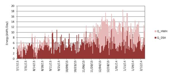
Figure 5. Daily thermal energy input for domestic hot water heating (bars are stacked).
