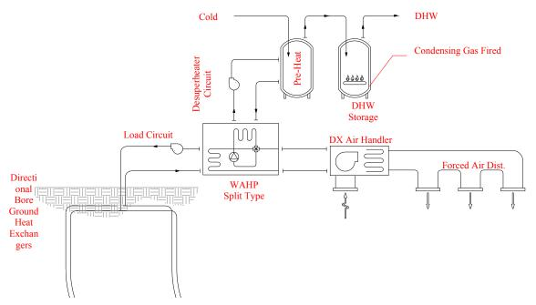
Figure 2a. Schematic of the water-to-air heat pump system at the Sacramento house. The system uses directional bore ground coupled heat exchangers. Desuperheater operates with heating and cooling.
