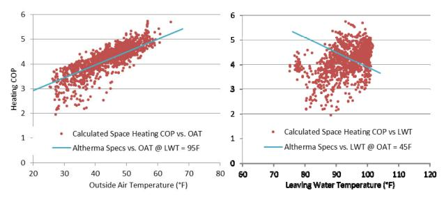
Figure 1. Measured COP of the Chico house AWHP in heating mode as a function of (a) outside temperature and (b) leaving water temperature. Manufacturer rated performance is also presented. (n = 1,383 15-minute intervals).
