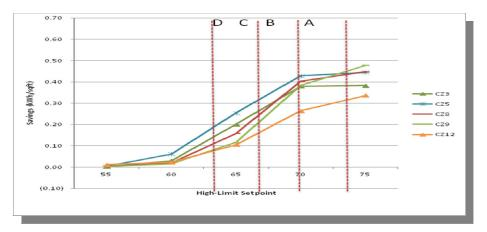
Figure 2. Economizer savings in different California climate zones, as a function of high-limit setpoint.
