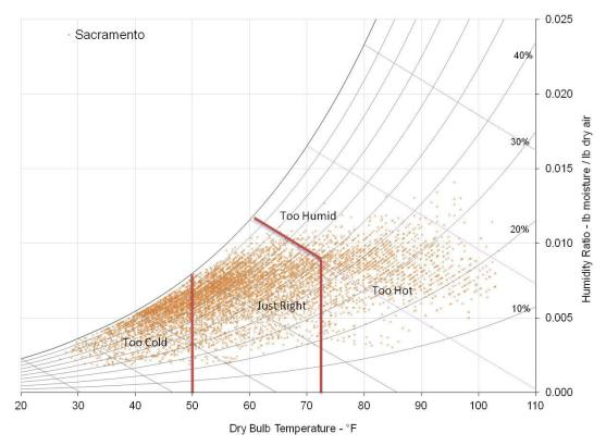
Figure 1. Climate conditions that are conducive and not-conducive to economizer savings.
