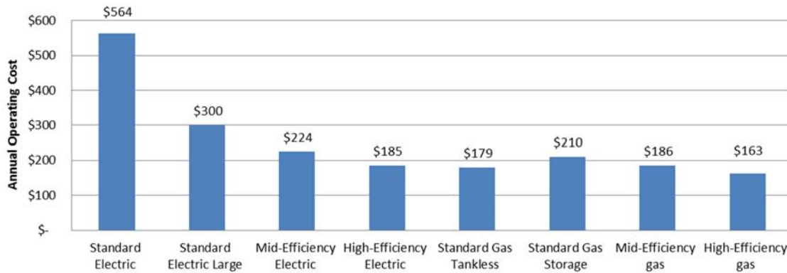
Figure 5: Average Annual Operating Cost of Water Heating for Prototype Home with Different Equipment Options
