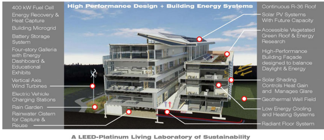
Figure 2. Illustration of building system. Source: SWBR Architect
