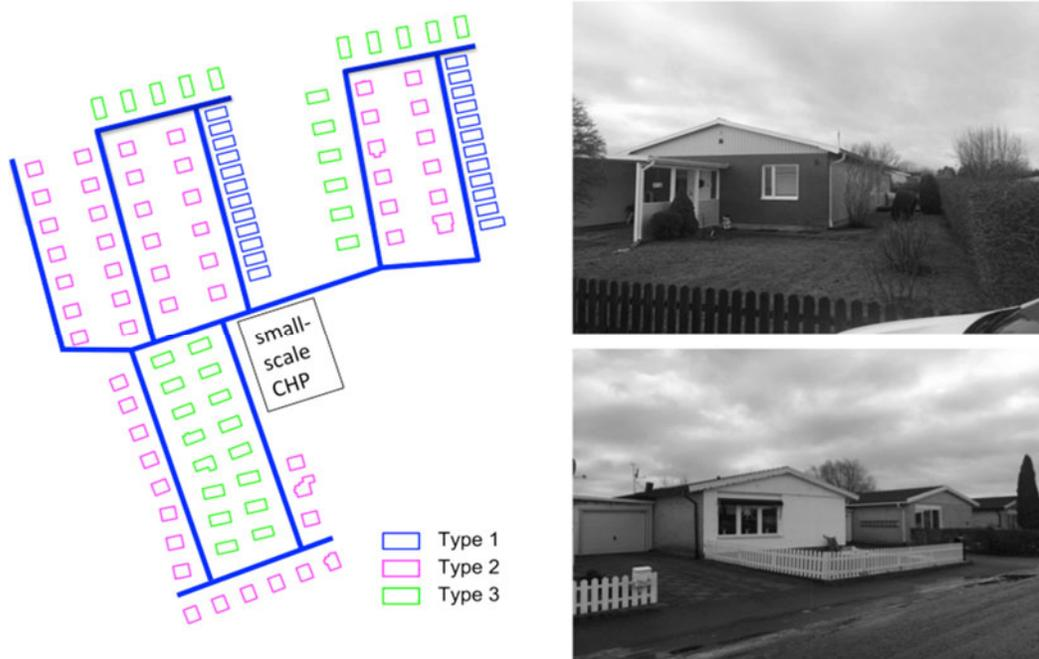
Figure 1. *Left:* The 111 studied houses grouped into three different types, main heat distribution pipes (thick lines), and possible CHP unit location in the area (white box). Possible layout used for heat loss calculations. *Right:* Typical single-family homes in Lövstalöt.
