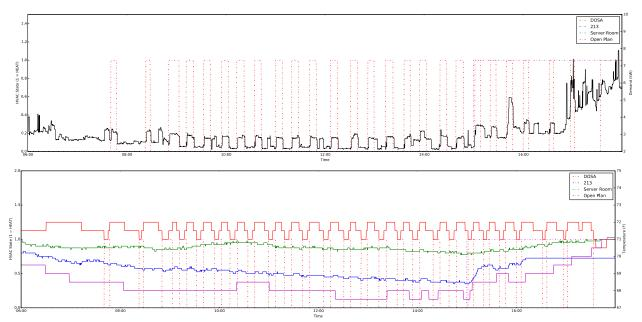
Figure 7. Dashed lines represent thermostat HVAC state. In the top plot, this is overlaid with the full building demand (solid line); in the lower plot, HVAC state is overlaid with the measured temperature for each thermostat (solid lines). We can visually identify that the "DOSA" thermostat dominates energy use during the plotted period.
