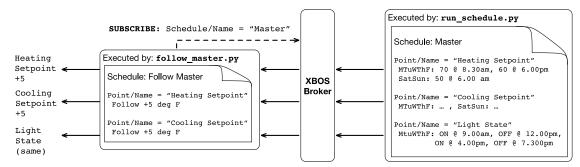
Figure 4. The "Follow Master" schedule subscribes to all outputs of the master schedule and selectively applies an offset. Here, the follow schedule adds 5 degrees to the heating and cooling set points of the master schedule before publishing them. The light state schedule point does not have an offset, so the follow schedule simply republishes it. The published points are identified with Schedule/Name = "Follow Master".
