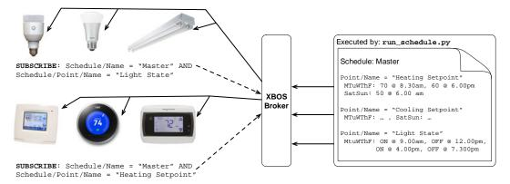
Figure 3. The basic communication pattern for how schedules are defined in XBOS. Devices (via their drivers) express a subscription query to the broker (dashed line), identifying which schedule(s) it is interested in. Schedules push their control decisions to the XBOS broker, which routes the current schedule settings to the relevant devices (solid lines).
