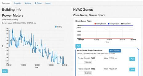
Figure 1. The XBOS Building Dashboard is autogenerated from the Building Profile and offers schedule management, device setting override, device and building status and visualizations.
