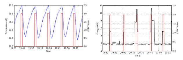
Figure 6. Left: Thermostat's reported HVAC state overlaid with reported temperature measurement. HVAC state of 2 indicates the thermostat is calling for cooling; 0 means the thermostat is "off." Right: Thermostat's reported HVAC state (cooling) overlaid with instantaneous building demand.
