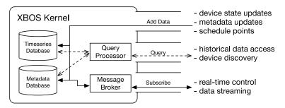
Figure 2. Architecture of the XBOS Kernel, which provides three interfaces to aid the construction of applications.
