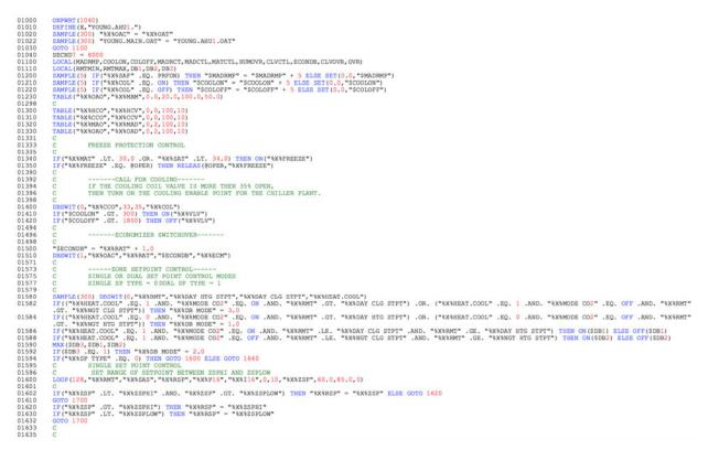
Figure 1: Page 1 of 5 of a traditional control sequence to control the normal operation of an air-handling unit using traditional vendor-specific control code.
