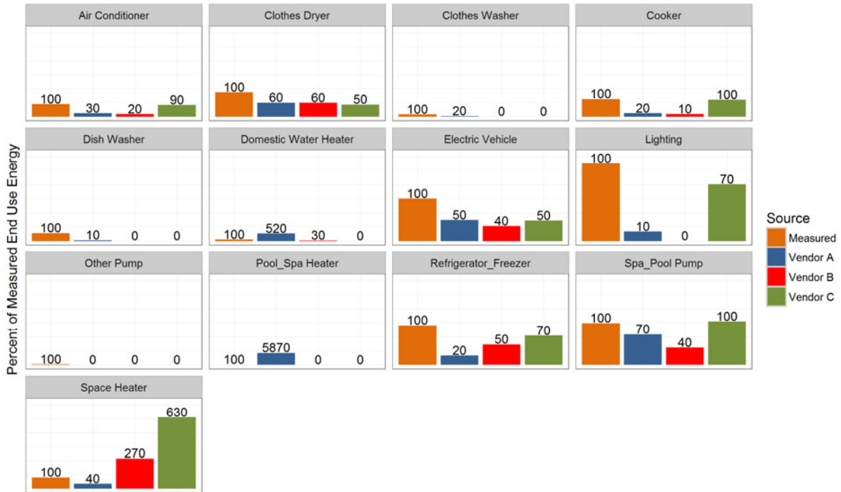
Figure 5. Percent of measured by end use and vendor (all test sites - December 2014 thru April 2015). All panels use the same scale.
