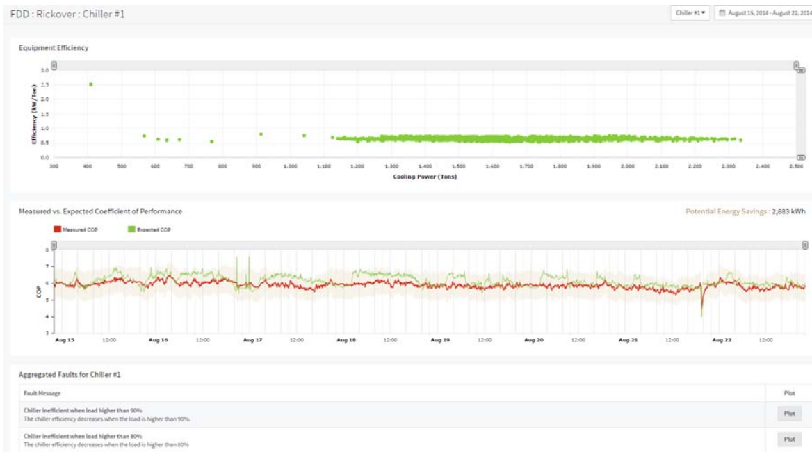
Figure 4. Screen shot of the fault detection and diagnostic features in the PlantInsight tool.
