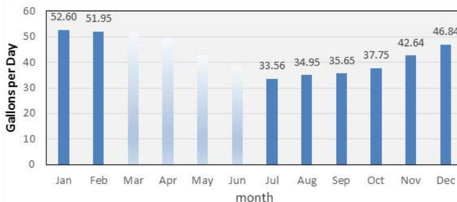
Figure 1. Daily volume of hot water utilized for the eight month testing period.
