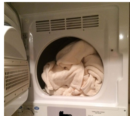
Figure 18. Partially-dried towels fill a dryer, reducing the air path so that they do not dry without a large added time.
