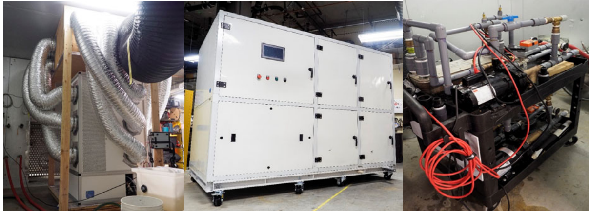
Figure 3. Nexajoule SWEC installed in the environmental chamber (left), Tsinghua SWEC in the WCEC laboratory (middle), and load rig for heating and supply return water (right).
