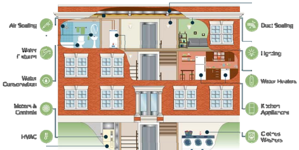
Figure 2. Ten building systems assessed by EZ Retrofit.
