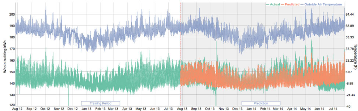
Figure 1. Actual and model-predicted energy data, overlaid with outside air temperature, for a 12-month training period and 12-month prediction period.
