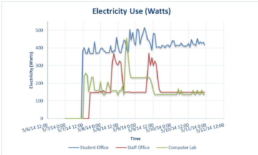
Figure 5: comparison of electricity use between workstation types
