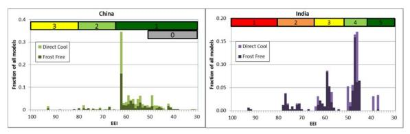
Figure 1. Stacked histograms showing the distribution of refrigerator models by energy efficiency index, separated by cooling method, in China (left) and India (right). Colored bars at top show the EL definitions for labeling programs in each nation, as well as our definition of an ultra-efficient level 0 for the Chinese market.
