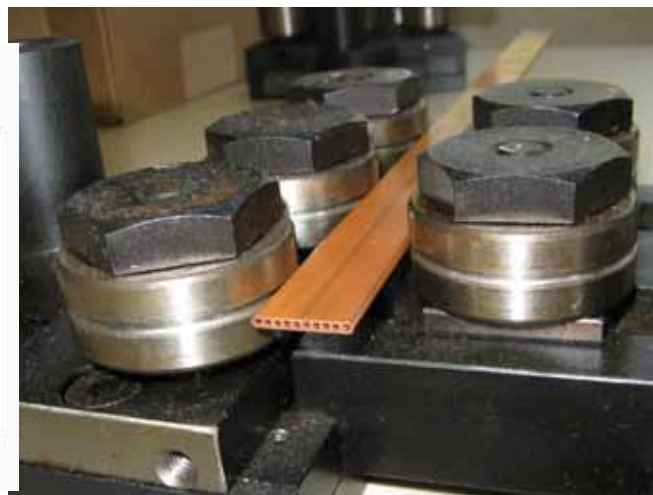
Copper minichannel tubes manufactured by Prof. Kraft, at Ohio University
