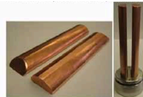
Copper minichannel tubes manufactured by Prof. Kraft, at Ohio University
