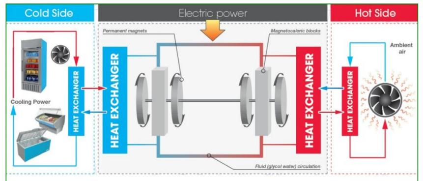
Replacing traditional fluid-compression refrigeration with longer-lasting magnetic refrigeration technology reduces energy consumption, eliminates coolant leaks, avoids damage to the ozone layer from chloro-fluorocarbons, and makes installation and service simpler.
