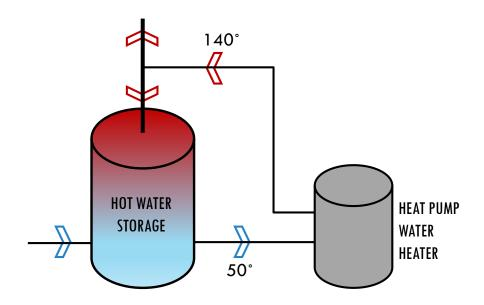
Heat the water up to usable temp in a single pass.
