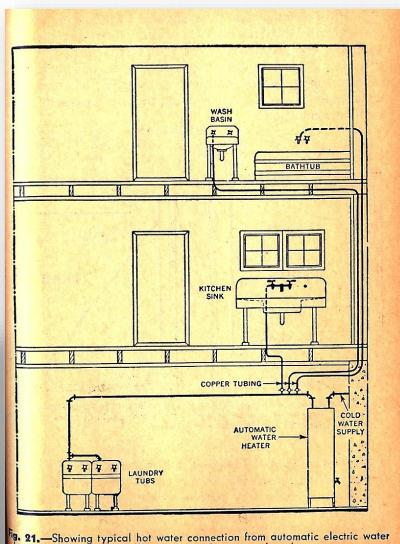
heater to fixture when small size copper tubing is employed.
