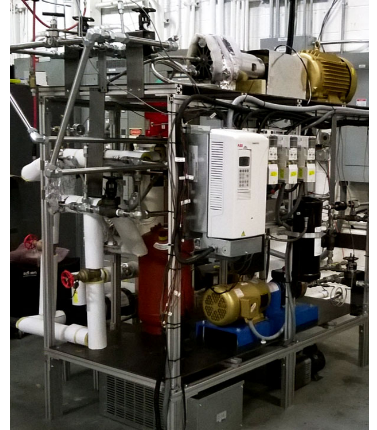
Tryden One System Alpha Prototype w/ Scroll Expander
