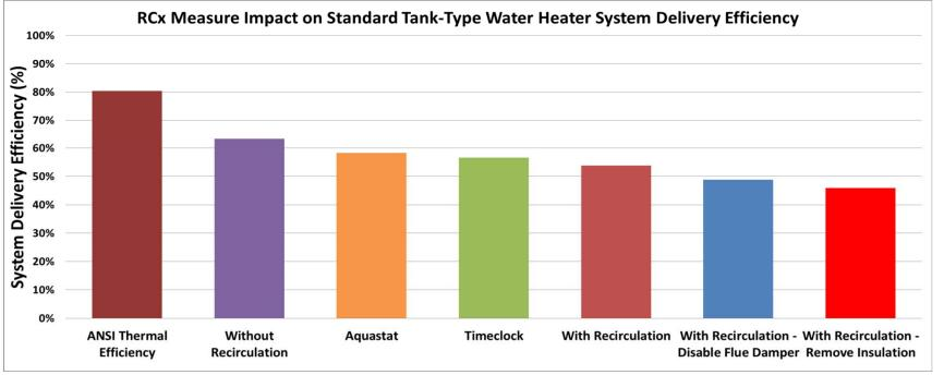
System Energy Performance Impact – RCx and Retrofit 24 hr. Draw Profile - Standard Efficiency Tank-Type Water Heater Insulated System
