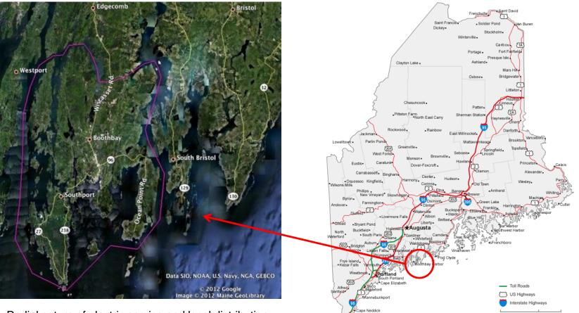
Radial nature of electric service and local distribution circuits on the Boothbay peninsula defines the electrical region for the Pilot Project – Total Peak load – Approx. 30 MW.
