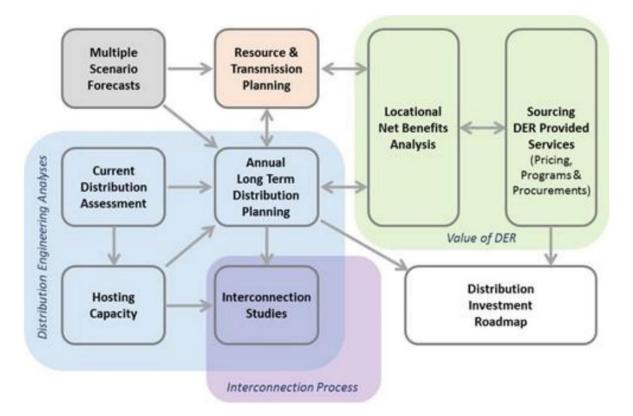
Figure 5. Integrated distribution system planning. *Source:* De Martini 2016.
