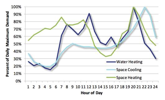
Figure 9. Illustrative hourly load profile for three residential end uses. Source: NWPCC 2016.
