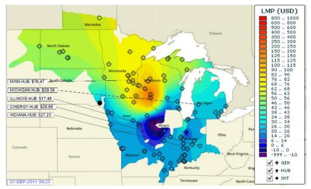
Figure 10. MISO real-time LMP on September 7, 2011 at 9:25 am. Source: EIA 2011.
