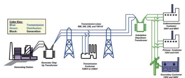
Figure 2. Structure of the electric system. Source: Hein et al. 2011.
