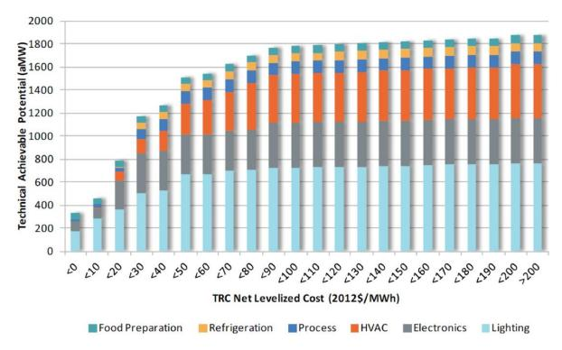
Figure 3. Commercial energy efficiency potential by 2035 by end use and levelized cost. Source: NWPCC 2016.
