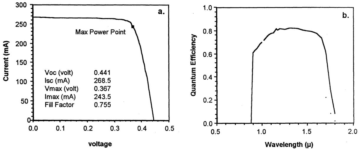
Figure 4. a.) Typical GaSb Cell Current-Voltage Characteristics at ~50x Solar Concentration b.) Typical Quantum Efficiency of GaSb Cell
