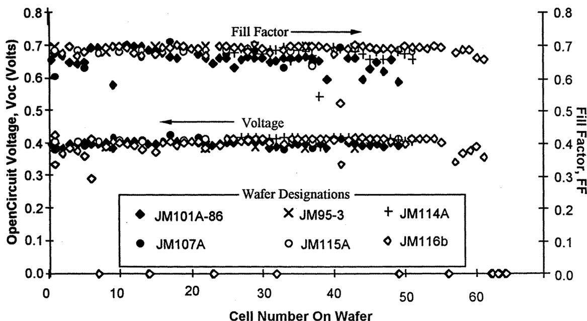
**Figure 5. Cell Fabrication Process Repeatability For Open Circuit Voltage (Voc) and Fill Factor (FF) Over Six Production Runs of Four Wafers Per Run**
