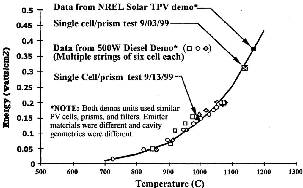
Figure 6: Comparison Of Measured And Theoretical TPV Power Out Versus Emitter Temperature
