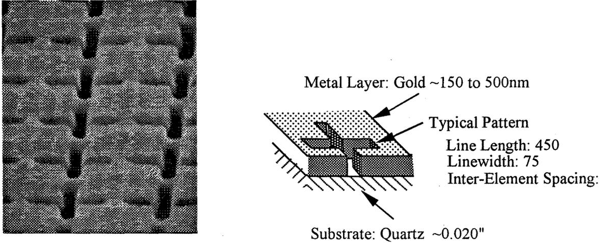
**Figure 2. Photomicrograph of Gold EDTEK TPV IR Filter With Schematic Diagram**
