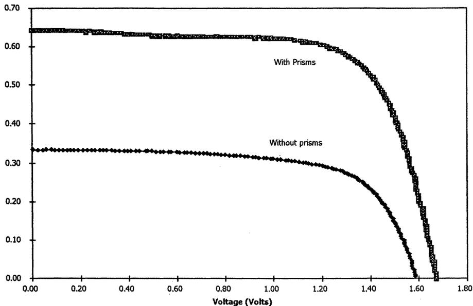
Figure 7. Measured performance of 4 series connected GaSb PV cells with and without concentrating prisms
