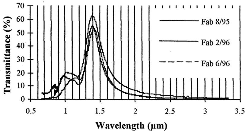
a. Batch to Batch Reproducibility of Fabricated Filters
