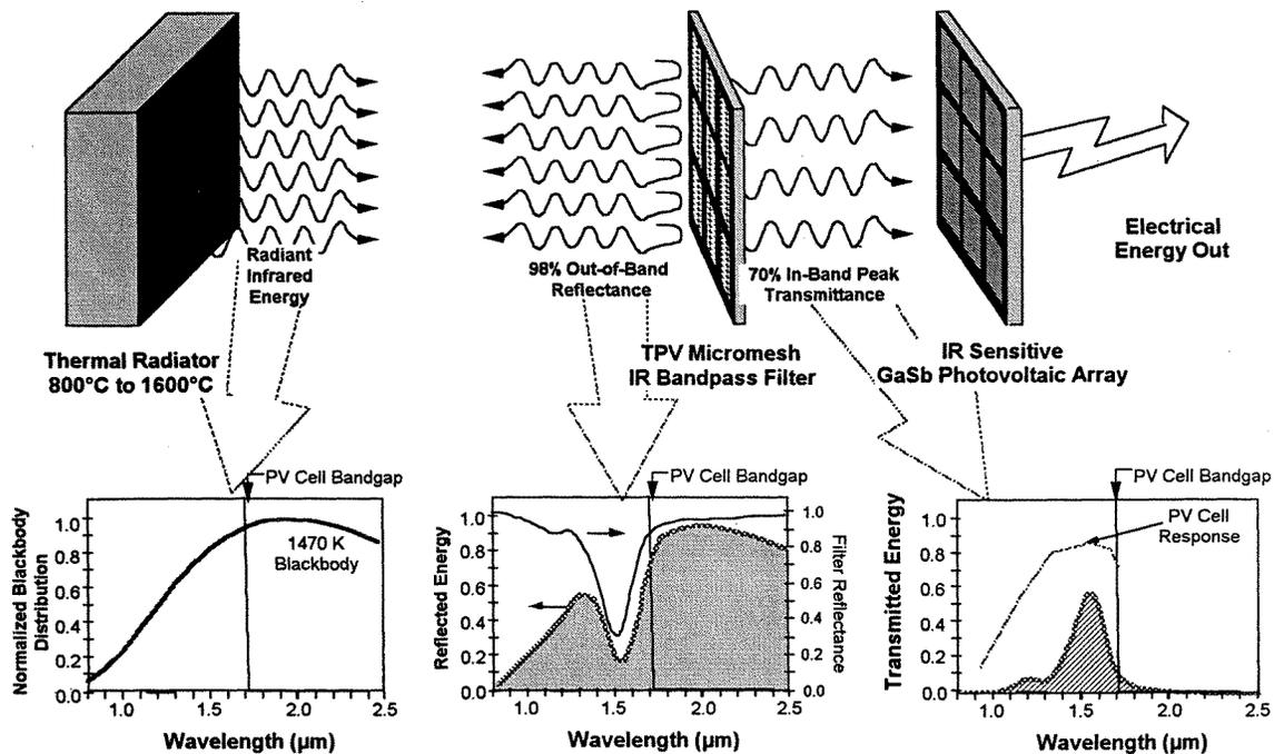
**Figure 1. Illustration of Basic TPV Conversion Process**
