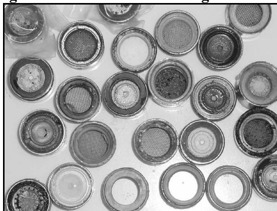
Figure 6. Old Aerators Missing Restrictors
