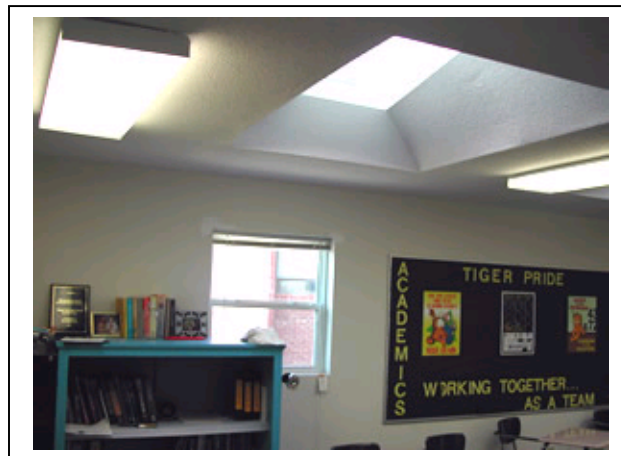
Figure 8. Daylighting from Overhead Skylights Inside Nc Experimental Classroom
