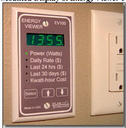
Figure 1. Wall-Mounted Display of Energy Viewer Feedback Device
