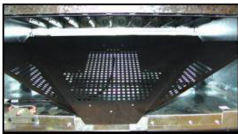
Figure 3. Delivery Chute with Improved Circulation (Left) and Tangential Variable-Speed Evaporator Fans (Right)
