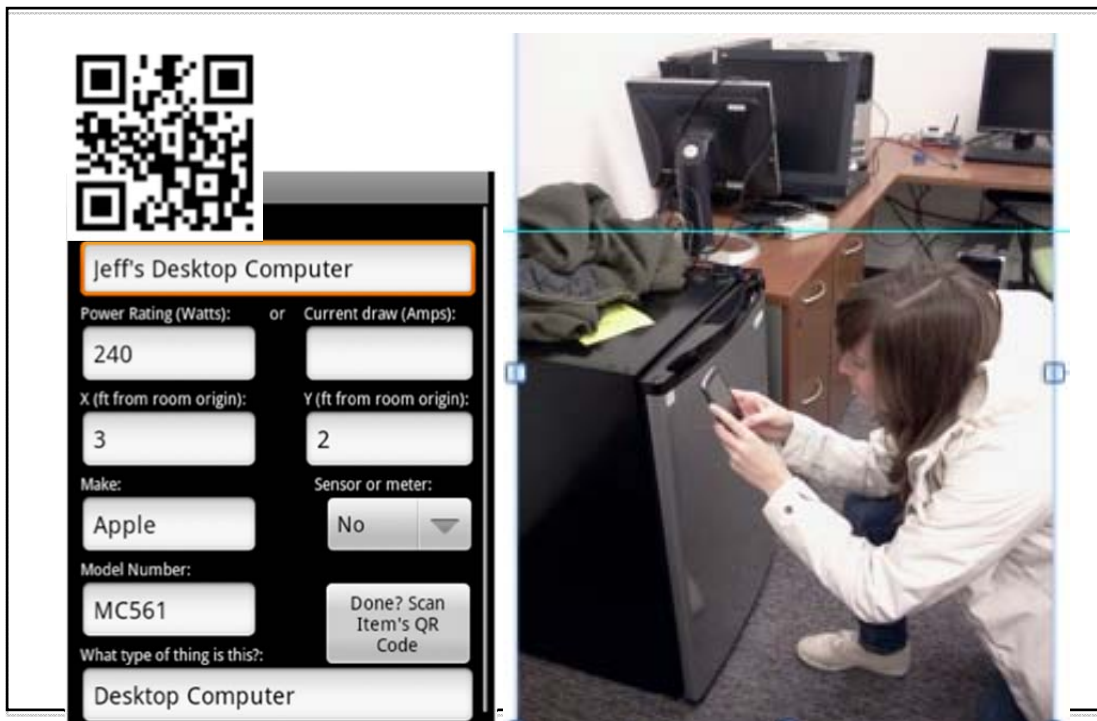
Figure 3. (Bottom right): Student Scans the QR Code (upper right) on an Appliance, and then Enters Information (bottom left), which is Streamed to a Database (photos Trager)
