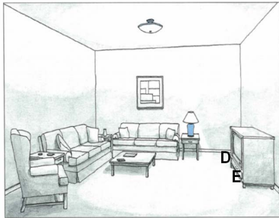
Figure 1. Three Dimensional Illumination of a Typical Living Room Illustrating Points D and E for Illuminance Measurement
