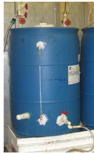
A biogas collector
