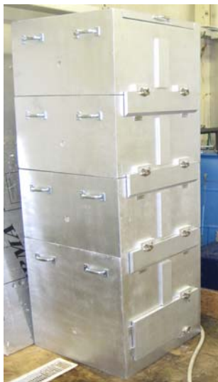
A fast aerobic bio-degradation reactor
