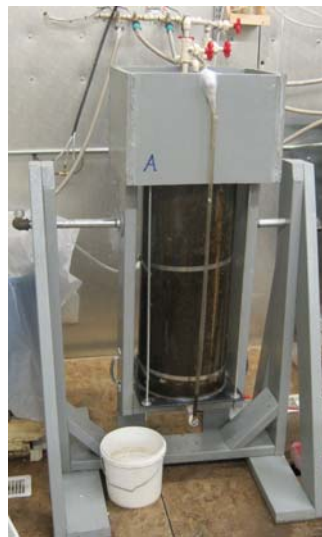
A cylindrical anaerobic bio-degradation reactor
