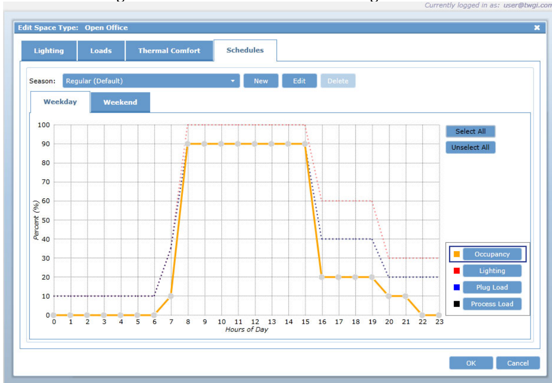
Figure 4. Schedules Tab of the Building Use Screen
