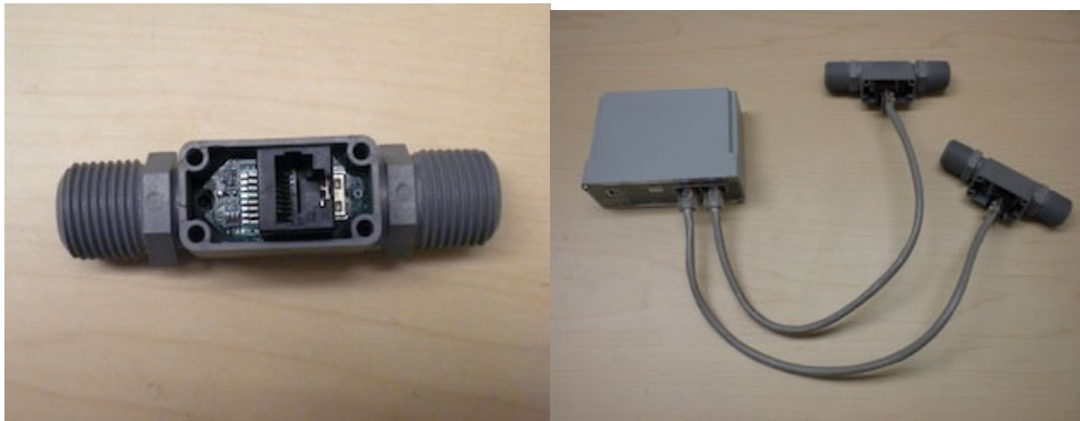
Figure 3. Fully assembled flow meter (left) and two flow meters per mote board (right).
