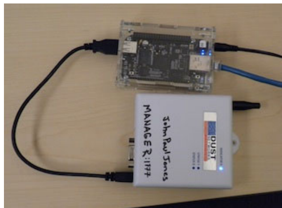
Figure 4. Manager mote and embedded computer.
